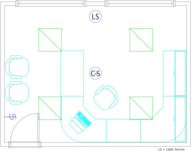
C-S = Ceiling-Mounted Motion Sensor
